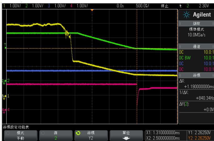
Figure 6 : How Power Failure Protection mechanism works?
